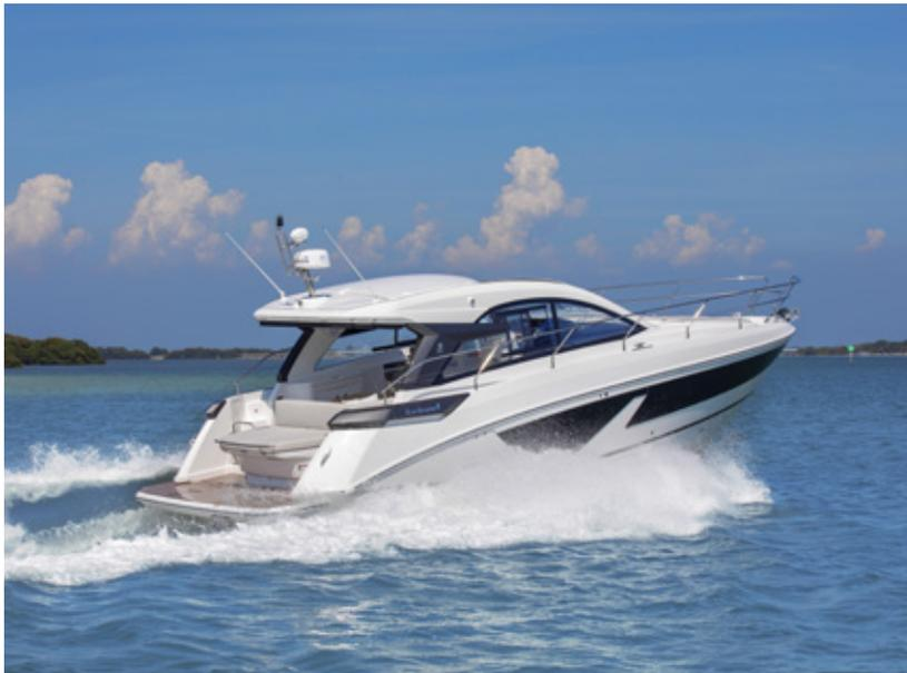
The Air Step® technology optimizes speed and stability by increasing the volume of air flow under the hull, leading to faster acceleration and reduced fuel consumption. The "Air cushion" effect is reinforced by rear pads, V-shaped steps further improving the boat's stability.
